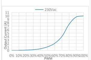
PWM Dimming Curve of Dim-to-off Version (logarithmic)
