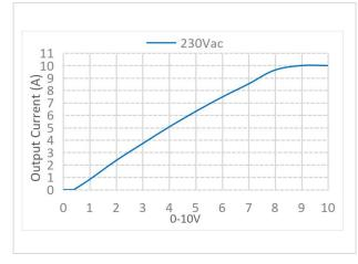
0-10V Dimming Curve of Dim-to-off Version (logarithmic)
