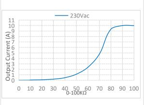
Input: 230Vac; output: 24Vdc/10mA (this data is measured by LEVITON dimmer and the chart is for reference only)
