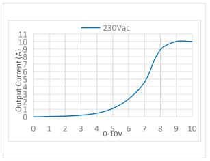
Input: 230Vac; output: 24Vdc/10mA (this data is measured by Lifud 0-10V dimmer and the chart is for reference only)
