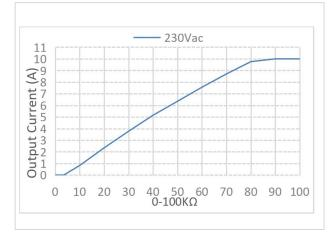
Rx Dimming Curve of Dim-to-off Version (logarithmic)
